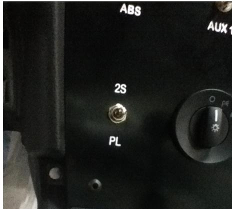
2. The RPM set point is adjusted by moving the toggle switch up or down. The RPM will change in 100 RPM increments. The user range for the launch control is 2000 rpm to 7750 rpm and the PCM will not allow any settings beyond these limits.
